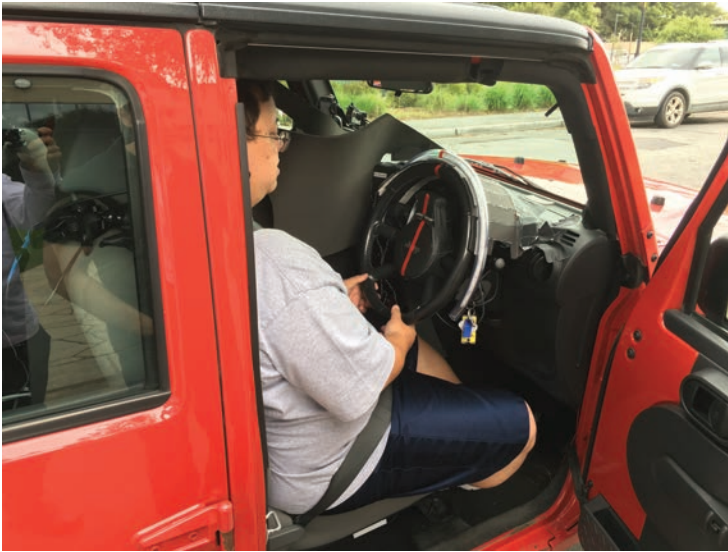
Figure 2.3: The RADDs platform at Stanford was used to explore automated driving — the vehicle’s steering wheel is on the right, and the driver is hidden from the participant by a partition. This setup encourages participants to imagine, or even believe, that the car is moving under the control of a machine agent.
