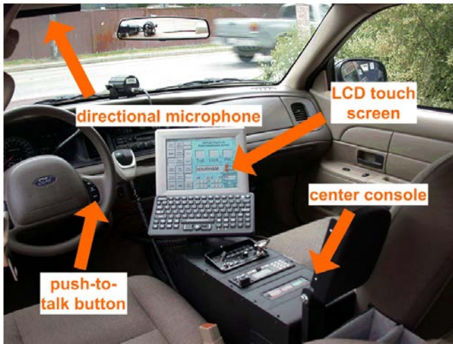
Figure 3.3: Project54 created a unique voice actuated computer system which integrated the control of in-cruiser devices such as lights and siren, radar, and video (Kun et al. , 2004; Kun et al. , 2003). The system also allowed performing voice driven data queries.
