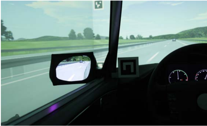
Figure 3.4: Ambient light display (purple light on the left) in the driving simulator at the University of Oldenburg (image by Maleah Maxie).
